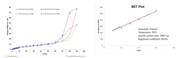
Comparison of Pt-SiO<sub>2</sub> toluene adsorption-desorption isotherms at 25 and 55°C (left). Determination of specific surface area using BET equation for toluene sorption at  $55^{\circ}$ C (right).
