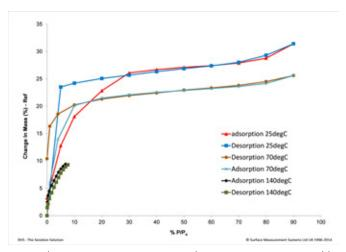
Comparison of 25°C water vapor adsorption-desorption isotherms for Mg-MOF-74 and TEPA-MOF-74. Mg-MOF and TEPA-MOF were prepared by Xiao Su & Lev Bromberg from MIT, Chemical Engineering. (Figure left). Comparison of 4A (Sigma Aldrich, 1/16inch diameter, 1-2mm pellets) water adsorption- desorption isotherms measured at 25, 70 and 140°C (Figure right). The large hysteresis at 25°C is due the fact that mass equilibrium at low P/Po was not reached.
