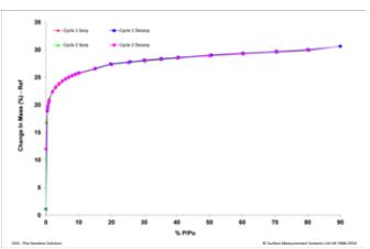
A10 (powder, Grace Chemicals) water vapor sorption at 40°C. Prior to sorption measurements A10 was *in-situ* degassed at 180°C under high vacuum of 10<sup>-5</sup> Torr for 480min and subsequently cooled down to sorption temperature of 40°C. Sample was regenerated between cycles using the same degassing conditions. Resulting water adsorption-desorption isotherms of A10 is shown on the right.
