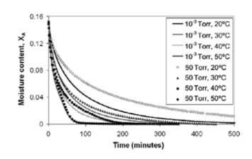
The effect of temperature and vacuum pressure is shown to provide information on dehydration kinetics of carbamazepine dihydrate.
