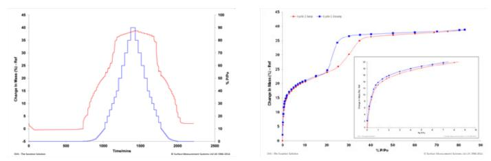
Zeolite Y benzene sorption at 25°C. Adsorption-desorption cycle showing benzene sorption kinetics (left) and corresponding isotherm (right) at 25°C. The inset shows the isotherm in the Henry region where pressure was increased by 0.2 % P/Po.
