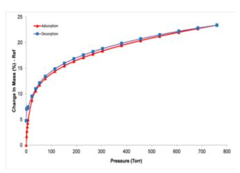
Mg-MOF-74 adsorption-desorption of  ${\rm CO_2}$  in the pressure range from 0 to 760 Torr 25°C.
