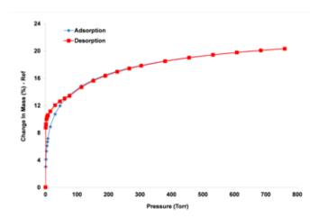
13X adsorption-desorption of  ${\rm CO}_2$  in the pressure range from 0 to 760 Torr at 25°C. 13X was in the form of beads having 1-2mm diameter.
