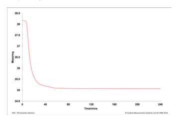
Drying curve of 13X zeolite, which was degassed  $\emph{in-situ}$  at 400°C and high vacuum.
