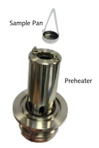
High temperature pre-heater for *in-situ* degassing/regeneration of samples up to 400°C. Temperature is measured by Pt-100 thermocouple, which is placed below the stainless steel sample pan.
