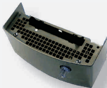
Photo: Slide-in cell cassette with sample cell carrier on top.
