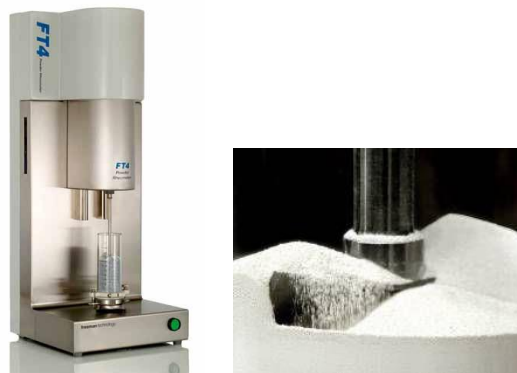
Fig. 2 FT4 Powder Rheometer (left) and dynamic flow test (right) ©Freeman Technology
