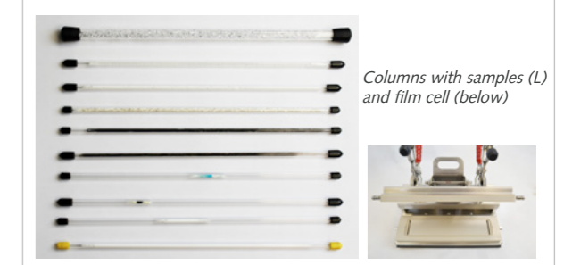
iGC-SEA straight column design - simple sample packing and column loading
